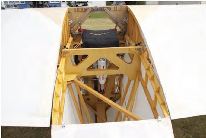
Ballistic Rescue System installed in aircraft.
